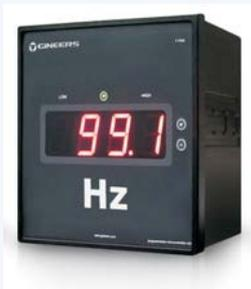
F4080 and F4100 are digital, fully programmable panel instruments from series 4080 and 4100. F4080/F4100 devices are used for frequency measurement 50/60Hz in electrical substations and power plants. They are powered by the measured AC voltage. F4080/4100 have potential-free contacts for remote signalization if measured frequency goes out of certain specified range (option "R"). F4080/4100 are designed to be mounted on boards in control rooms in electrical substations.
