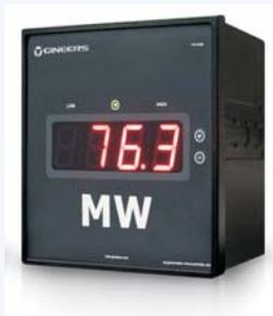
VA(R)4080 and VA(R)4100 are digital measuring, fully programmable panel instruments from series 4080 and 4100. VA(R)4080/4100 measure signed active (VA4xx0) and reactive (VAR4xx0) electric power in electrical substations and power plants. VA(R)4080/4100 are designed to be mounted on boards in control rooms in electrical substations.
