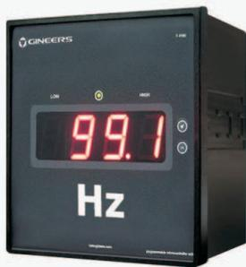
F4080 and F4100 are digital, fully programmable panel instruments from series 4080 and 4100. F4080/F4100 devices are used for frequency measurement 50/60Hz in electrical substations and power plants. They are powered by the measured AC voltage. F4080/4100 have potential-free contacts for remote signalization if measured frequency goes out of certain specified range (option "R"). F4080/4100 are designed to be mounted on boards in control rooms in electrical substations.
